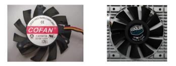
3. If CPU fan does not rotate, replace the whole CPU assembly with E5072-62090.
