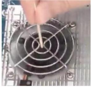
2-1. If CPU fan is COFAN, replace CPU fan with a new one (3160-4452) for repair.2-2. If CPU fan is COOLER MASTER, replace CPU fan with a new one (3160-4518) for repair.
