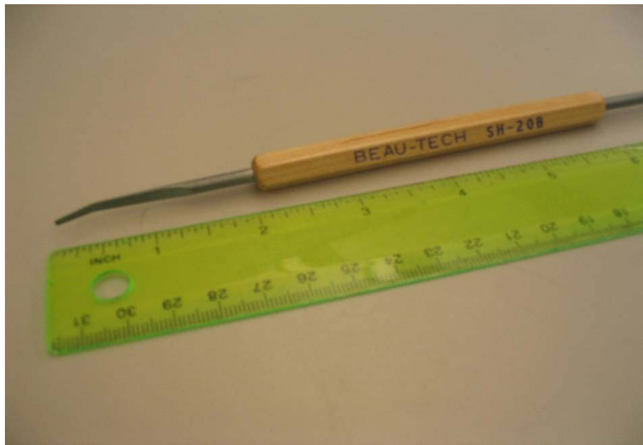
Figure 3 – generic tool to re-insert power supply connector
