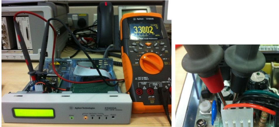
(Picture 3: Measure output Voltage with Digital Multi-meter)
