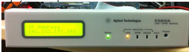
(Picture 5: Turn on the E5810 to ensure the IP display in the screen and fault LED OFF)
