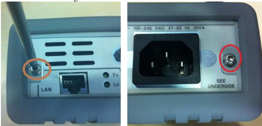
(Picture 2: Unscrew the screw using Trox T8 Screwdriver)
