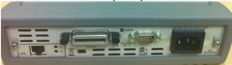
(Picture 1: Remove the Bumper attach to E5810 if any)
