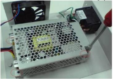
7. The protective cover is now successfully assembled. Put and align the whole power supply back to the SLU and then fasten it with the two screws.
