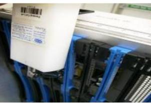
Figure 2. Jointed Test Finger touches the internal power supply of E6198A Switch/Load Unit.
