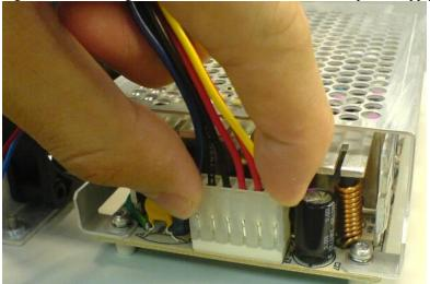
5. Plug in the new power supply cable (E6170-61601) mating connector housing to the power supply output connector. Ensure that the connection is tight.
