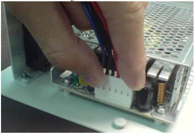
6. Put and align the whole power supply back to the SLU and fasten it back with the two screws.
