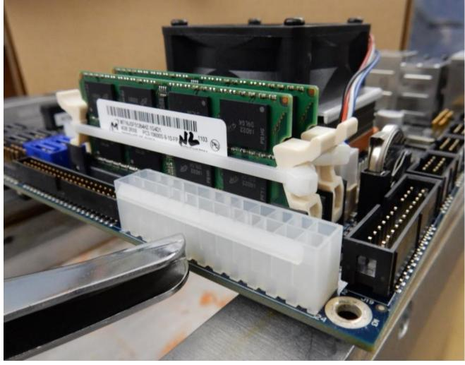
5. Inspect the underside of the Embedded PC and add 4x N5101-20005 or 1x E7515-40021 if not already installed.
