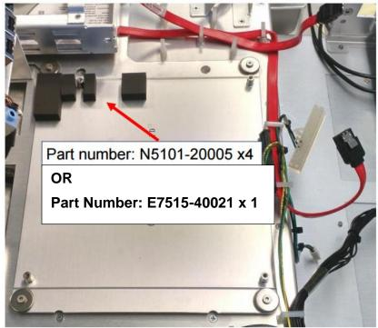
6. Re-install the Embedded PC and attach cables. Add cable ties, 1400-3557, to the USB Cables
