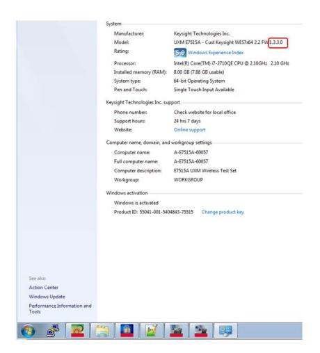
If the revision number shown is below 1.7.x.x (i.e. like the above image), please contact your Keysight Technical Support engineer to check your instrument and upgrade the Windows Recovery image at your next calibration.
