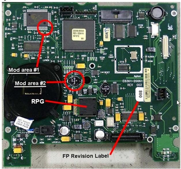
Refer to Figure 1 for the two modification areas to be addressed. Note that while this picture happens to show the FPI board completely removed from the front frame assembly, this is not necessary to perform the required modifications.
