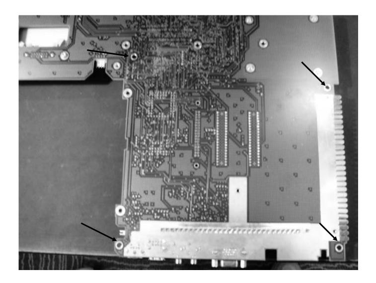
Use washers (3050-2187) with long mounting screws when re-assembling.
