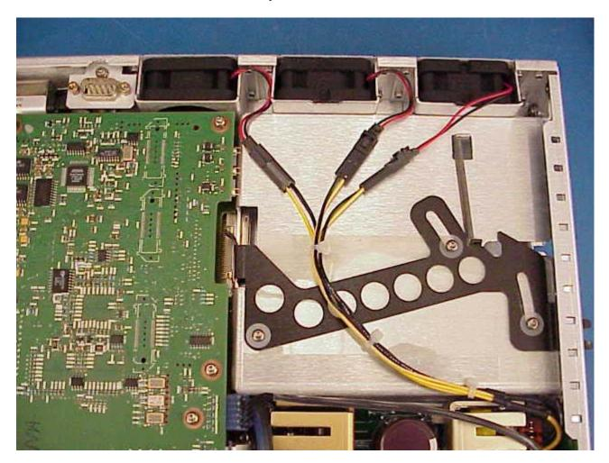
Shown here are the 5V fan connections.
