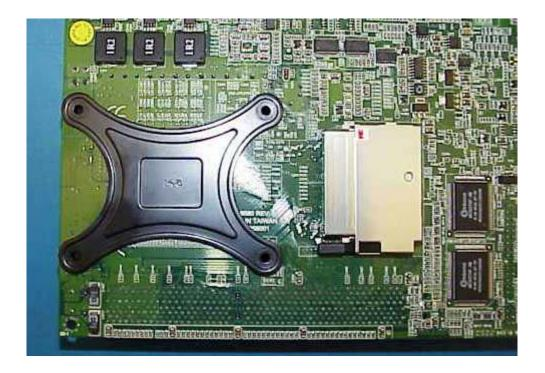
Turn the assemblies over, place the cooler fan on top of the CPU and tighten the screws at each of the corners in a crossing manner. (Upper left, lower right, Upper right lower left.)
