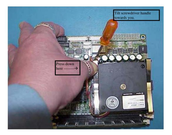
Repeat the process for the second clip. Once the clips are removed, the fan can be removed from the mother board. Discard these pieces as they are not required for the replacement.
