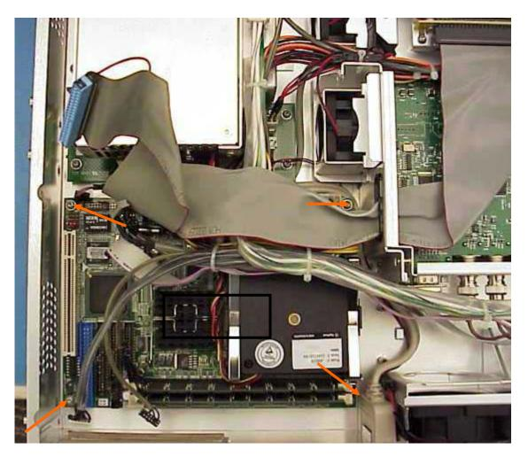
With the screws removed, you can now lift the mother board out of the chassis. It is now ok to remove the two power cables from the mother board.
