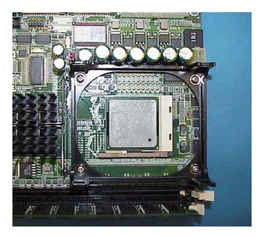
Open the packet of silicon heat sink material. Apply very sparingly. You only need to rejuvenate the original silicon on the top of the processor, DO NOT over-apply as this can cause a problem with the heat transfer as well.
