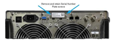
3. Loosen the eight captive screws indicated in the below figure. These screws are not removable; loosen them until they spring free from the chassis.
