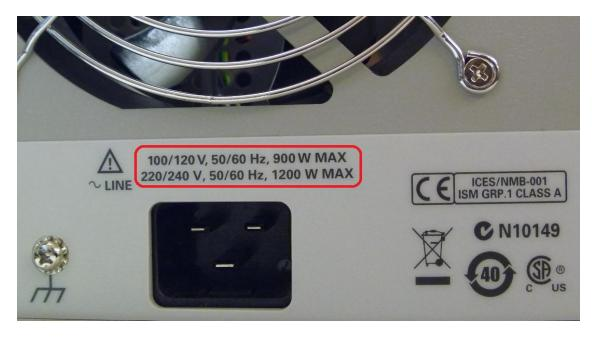
If the power supply was replaced/upgraded, the chassis will not have any "LOW POWER" sticker on the front panel and the back of the chassis will have power rating as shown below.
