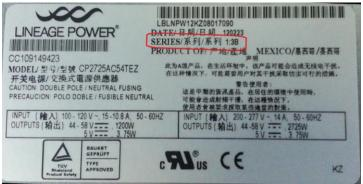
Replace power supply module to avoid system reset due to line voltage dropout issue
