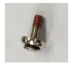
Replace the screws on the chassis carry handle. Tighten the handle screws to 23-25 kgf.cm (20-22 inlbs). Perform the same step to replace the screws on the second carry handle on the other side of the chassis.
