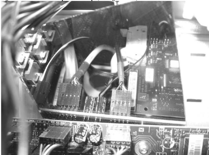
A mirror was used to aid in showing how the connectors begin to disconnect. Notice the gold pins visible under the connector on the left; the connector on the right was re-seated to show the contrast following the single drop. There are two known instances where one or more of these three cable connections have disconnected completely during transit
