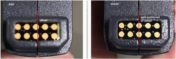
Please return defective probe amplifier to service center for repair.
