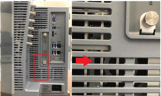
This is how the new fanless power supply will look like. You can see the edge of the PCA and components through ventilation hole.:
