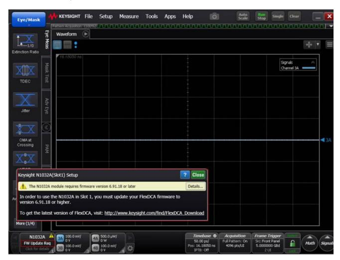
To update FlexDCA software, download from <a href="www.keysight.com/find/flexdca\_download">www.keysight.com/find/flexdca\_download</a> and install. While only the indicated version is required, updating to the latest version is recommended.
