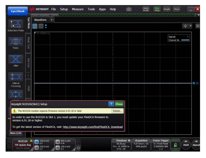
To update FlexDCA software, download from <u>www.keysight.com/find/flexdca\_download</u> and install. While only the indicated version is required, updating to the latest version is recommended.
