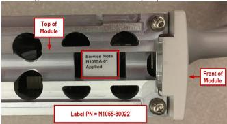
2) "N1055A-01" shall be added to the comments field of the unit's memory. When applicable, the N1055A test code will ask if this service note has been executed and update the comments field accordingly. Select 'Yes' if new-design boards are installed:
