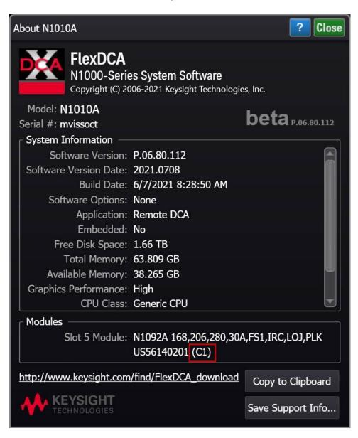
Note that the "C1" annotation is NOT used for units with option 40A because all units have the improved ER calibration.
