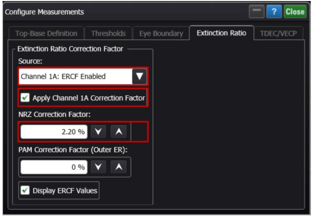
No ERCF is available for <u>PAM-4 signals</u> because the Outer ER measurement was previously uncalibrated.
