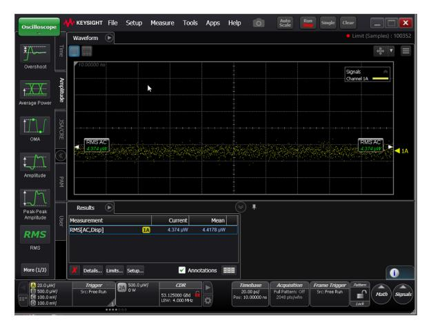
c. Compare the Mean value displayed to the specification table shown below. If the displayed noise is above the value in the table, the noise was impacted. You may send the unit back to Keysight for re-calibration and adjustment. Alternatively, you may try to perform a "User Optical Calibration" as described in the following section below.
