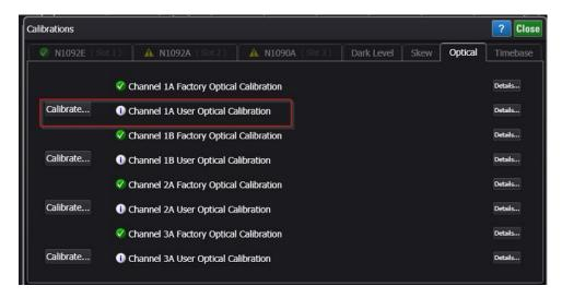
A CW multimode optical source is required for this step. Instructions on how to perform an Optical Calibration can be found in the FlexDCA Online help at the link below:
