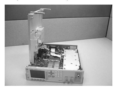
Disconnect the four connections shown.
