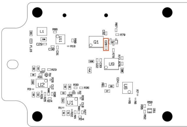
If this capacitor has been removed, no further action is required. Reassemble the ECal module.
