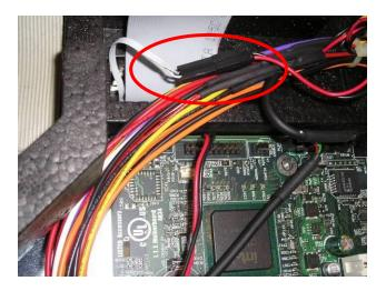
Now cautiously reseat the cover of the unit by carefully sliding it into the slots of the front frame, but do not fasten the screws (yet).
