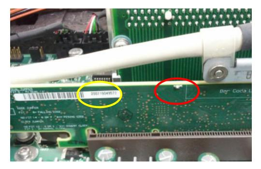
The board has a fuse on top (red circle) and a serial number (yellow circle) starting with 200... In the case above it is 200719049572)
