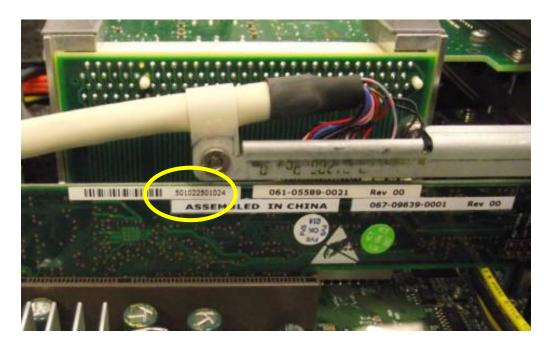
The board has a serial number (yellow circle)  $\pmb{NOT}$  starting with 200... In the case above it is: 501022501024.
