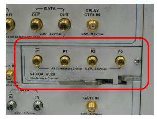
Due to mechanical problems (physical thickness of the front plate) there may be connection problems, i.e. the connector at the other end of the plug-in does not full insert into the connector inside the N4903A/B. The next picture shows the connector at the other (inserting) end of the N4903A/B-J20 plug-in.
