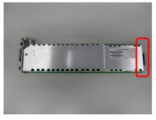
Therefore we may have to exchange the front plate and replace it with one that has the correct physical dimensions.
