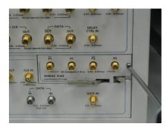
Turn on the N4903A/B and check whether the plug-in is recognized correctly.
