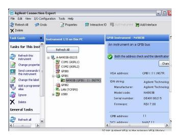
Identify the **GPIB1 interface** and notice the line underneath: "N4903B (GPIB1::11::INSTR).
