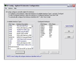
**3.** On the left side, under "Available Interface Types" you should see a line "Internal Instruments".
