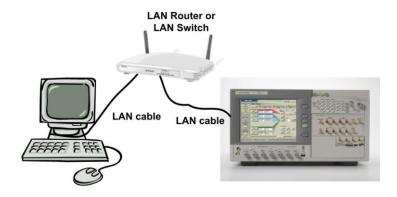
The Agilent IO Libraries have the task to route the network packets that contain the commands and that come from the external PC controller over the network to the N4903B software and hardware.
