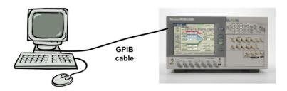
On a GPIB bus there can be several "slaves" but only one "master", which, in the case above, would be the external PC controller connected to the GPIB bus. However, in the noted serial number range of the N4903B product there may be the cases that the N4903B may act as master, too.
