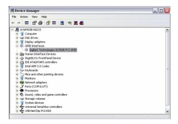
If you do not see the card or the card show a "yellow bang" in the window above, the card itself may be dead or not seated correctly in the PCI slot of the internal PC. Please check.
