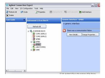
Identify the **GPIB2 interface**. It has a red cross and it shows an error in the right half of the screen. That is normal in this case. Do not get confused by that!
