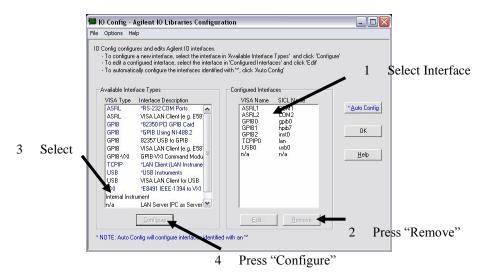
5. Select "Internal Instrument" in the window above and press "Configure" (step #3 and #4).
