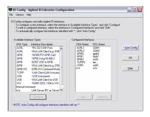
**5.** On the left side, under "Available Interface Types" you should see a line "Internal Instruments".
