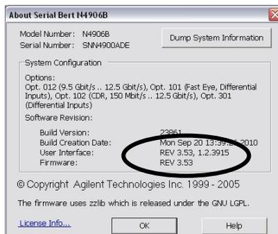
3. If the currently installed version is less than REV 3.53, please download the latest software from the Agilent website (<http://www.agilent.com/find/SerialBERT>).
