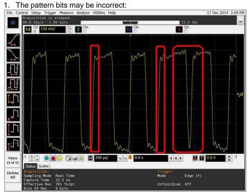
In the picture above, the set pattern is a divided clock (00001111). Each sequence of 0's and 1's should be the same length, and they are not. Incorrect bits are circled in red.
