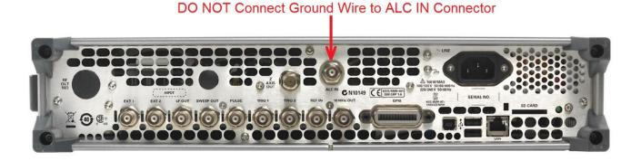
The typical failure symptoms of an instrument that has been exposed to this is the failure of Self Tests 407, 1107, 1108, 1112 (some or all of these). The parts that will be damaged are on the A7A1 Microwave ALC Control board, so the power level accuracy test will most likely fail as well.
