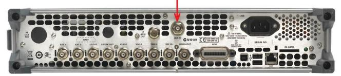
The typical failure symptoms of an instrument that has been exposed to this is the failure of Self Tests 407, 1107, 1108, 1112 (some or all of these). The parts that will be damaged are on the A7A1 Microwave ALC Control board, so the power level accuracy test will most likely fail as well.
