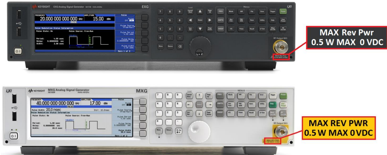
Figure 2 – X-Series \mu Wave Signal Generator Maximum Reverse Power Level Labels
