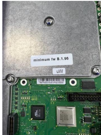
Figure 3 – Location of label on the RF assembly
