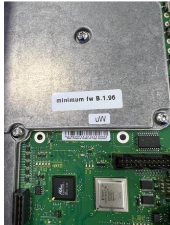
Figure 3 – Location of label on the RF assembly
