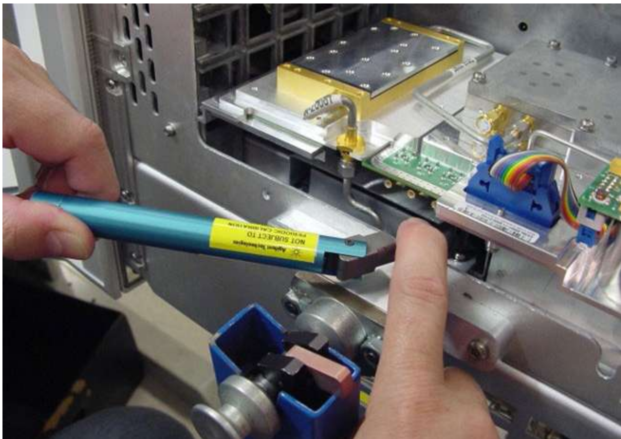
f. Secure screw using the modified 10 lb-in breakaway wrench.
