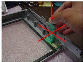
Must never handle or pull the touch screen up from the Front Frame by using the cable. The cable is very fragile and can cause the traces to fracture.
