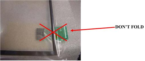
Never lay down the touch screen with the cable folded under. This will create a crease in the cable and fracture the conductors within the cable.
