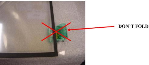
Never lay down the touch screen with the cable folded under. This will create a crease in the cable and fracture the conductors within the cable.
