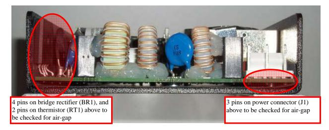
If there is an air-gap, the power supply can be re-fitted to the chassis and returned to the customer after being tested in accordance with the procedures outlined in the above mentioned service manual.
