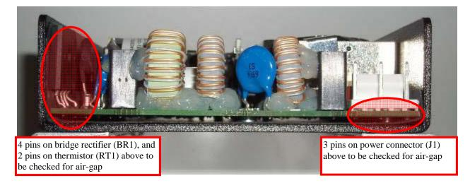
If there is an air-gap, the power supply can be re-fitted to the chassis and returned to the customer after being tested in accordance with the procedures outlined in the above mentioned service manual.
