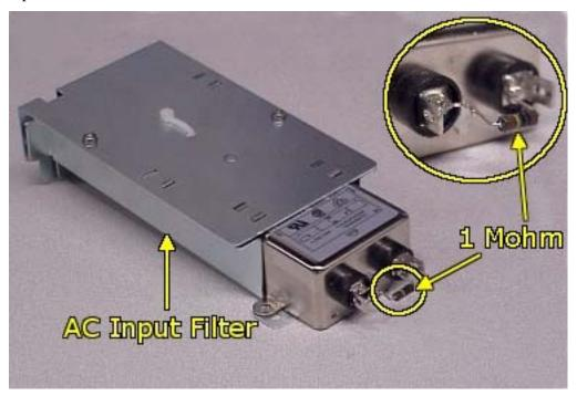
Begin by shorting the load terminals of the AC Input Filter Module to discharge the internal capacitor.
