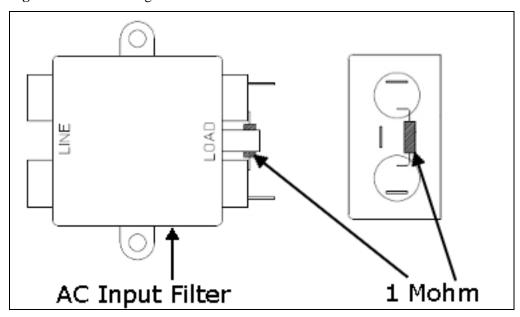
**Figure 2.** Demonstration of soldering the 1Mohm bleeder resistor across the load terminals of the AC Input Filter Module
