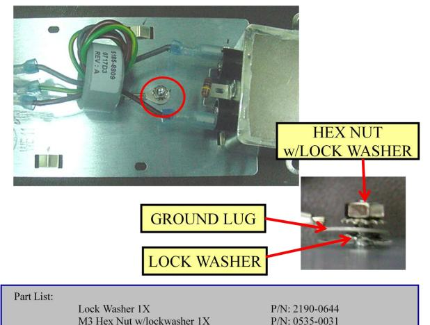
Figure 2. Demonstration of properly installed safety ground connector
