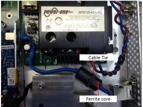
c) Detached the LAN cable (N8262-60203@blue color) from PPMC Assembly (N8200-60002) and rear panel LAN port (1253-7195).
