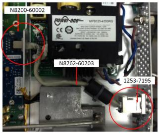
f) Ensure LAN cable connection to PPMC Assembly (N8200-60002) and to rear panel LAN port (1253-7195) are latch properly.
