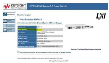
Figure 1: Serial number is "0" in WebUI
