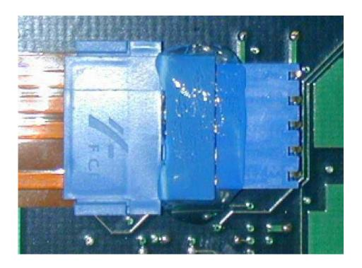
Fig 3 – Connector J10 with RTV added
