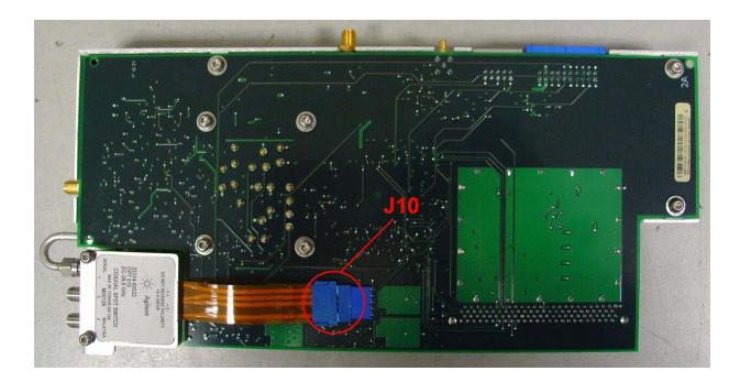
Fig 1 - A3 Assembly Showing Location of Connector J10
