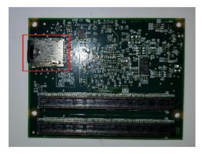
c. Using an Exacto Knife remove the Epoxy bridge holding the SD Card into the SD card socket.
