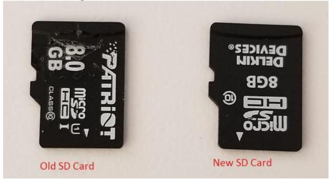
g. Insert the NEW SD card into the SD card socket and press it in until you hear a click, then release. The SD card is now locked in the socket.
