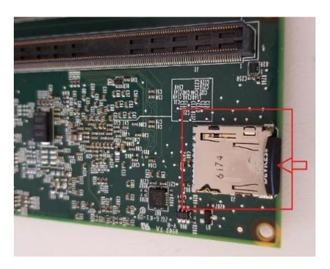
h. It is now necessary to add a small amount of RTV (part number 0470-0450) to bridge the SD card to the SD card socket. Using a wooden Q-Tip place a small amount of RTV on both the SD card and the socket.
