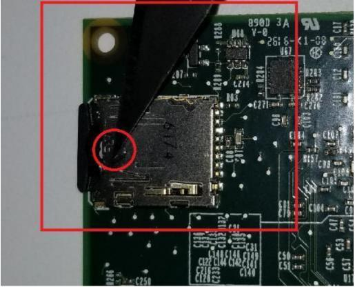
d. Use caution to not damage the socket or other parts of the CPU board.e. To remove the SD card, press the SD card slightly in towards the socket, it will click and then release to remove the SD card. Remove any extra epoxy that may be left.
